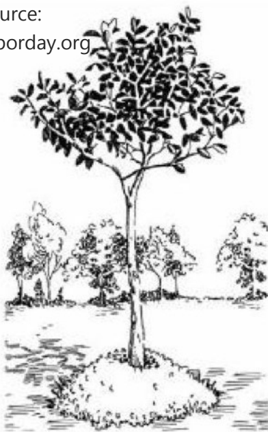
Improper Mulch Root flare buried & Mulch piled high up against the trunk
